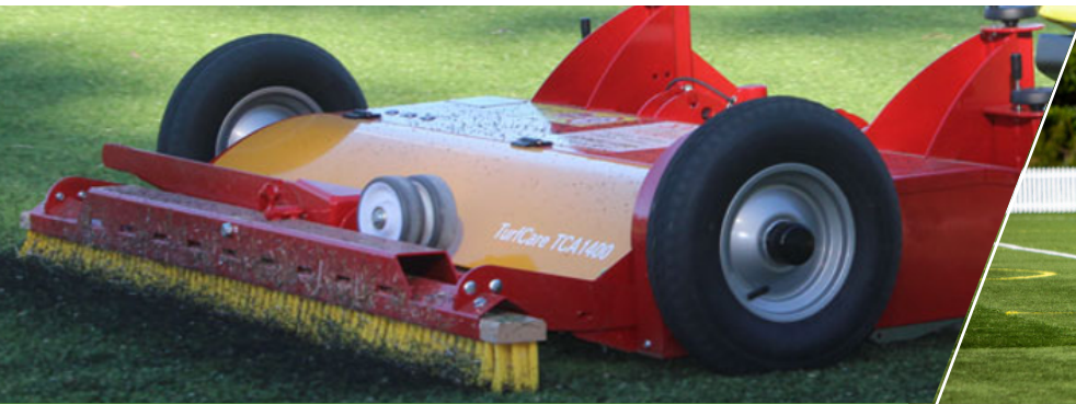
SMG TCA1400 in action during a Groom Service of a long pile field.
